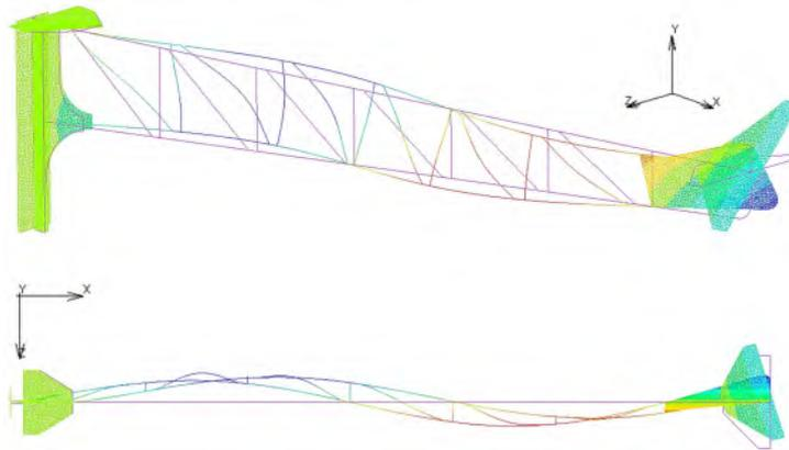
Figure 4.12 – 3d-view and top view of the deformed and original states of the structure for the 5<sup>th</sup> mode, obtained with the numerical reference model (fully rigid connections). The colours correspond to different quantities of out-of-plane displacements along the  $z$ -axis.
