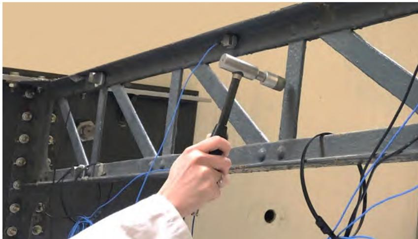
Principle of vibration tests on the tested lattice girder (Picture by H. Franz).
