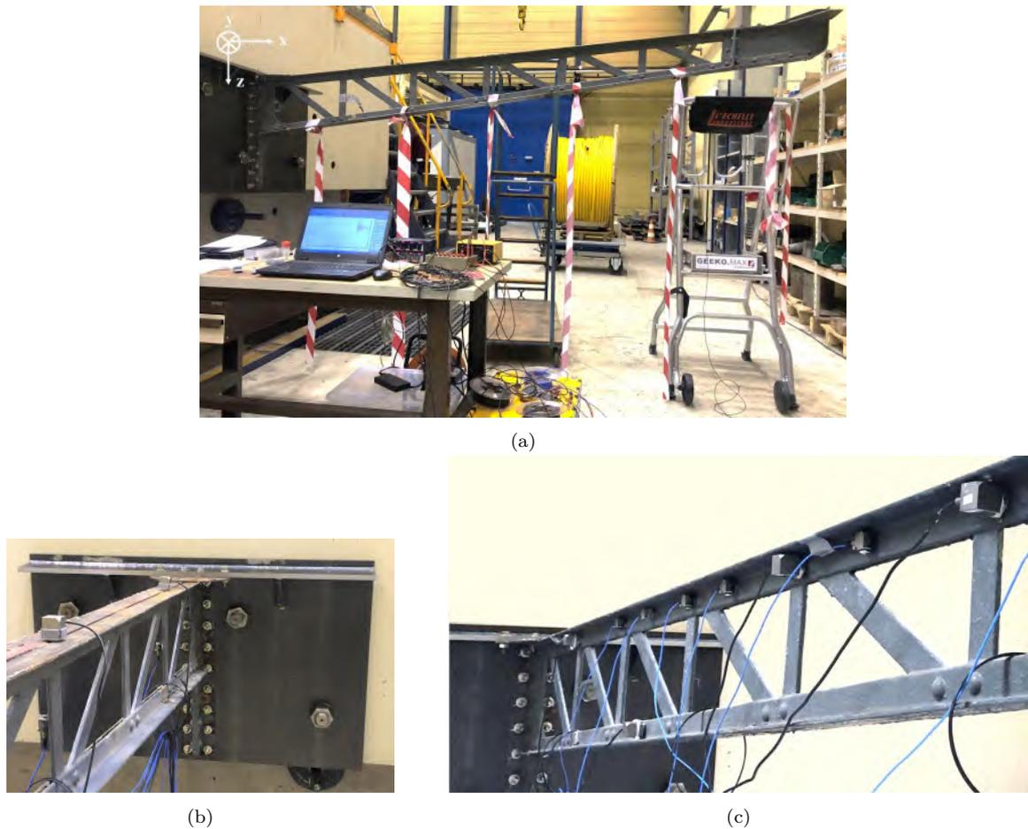
Figure 4.4 – Experimental setup in the laboratory: (a) global view; (b) fixation system of the girder; (c) girder instrumentation.
