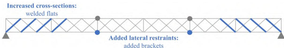
Figure 2.17 – Principle of the strengthening measures implemented on the lattice purlins of the train shed of Montauban, France.
