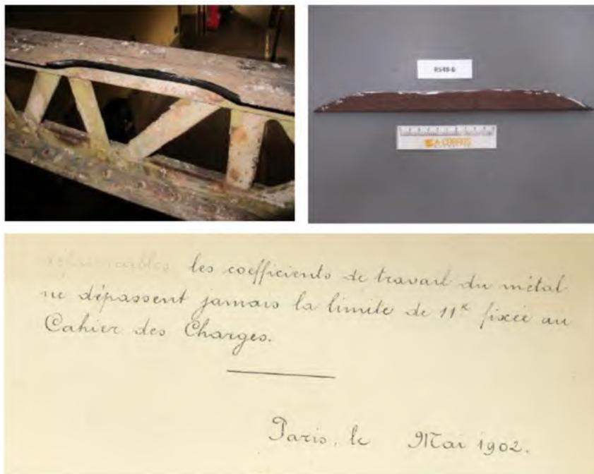
Top: specimen for material testing (Picture from the survey of the station Gare de Marseille St-Charles by A-Corros, 2017). Bottom: historical design report of the train shed of Bédarieux, 1902.
