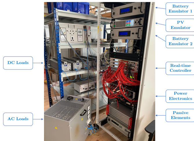
Fig. 4: Real-time PHIL setup consisting of PV emulator, loads, Real-time controller, SiC-MOSFETs, passive components and battery emulator
