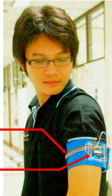
Fig . 5 : Prototype of a wearable e-nose based on using the flexible inkjet-printed chemical sensor array integrated in ZigBee wireless network. Reproduced from ( Lorwongtragool et al., 2014 )
