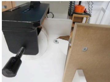
(b) Transverse tear-out of particle board
