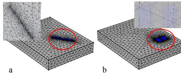
**Figure 1.** The meshing of the 3D model of a concrete slab (700x900x150 mm<sup>3</sup>) with a) the resistivity probe and b) the capacitive electrodes.
