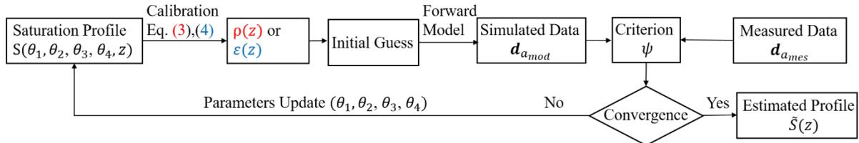
**Figure 2.** Scheme for the estimation of the saturation depth profile (parameters  $\theta_i$ ) from apparent resistivity or permittivity measurements.
