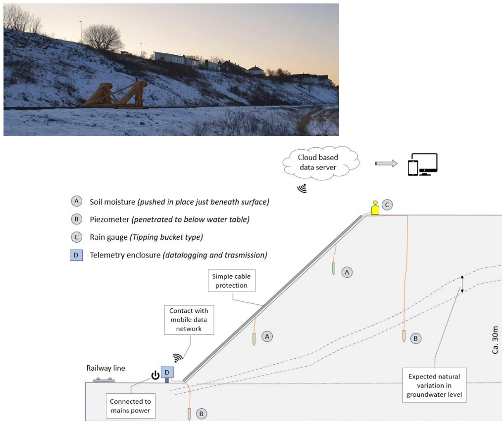
Figure 8. Overview slope, Bodø central station and pilot monitoring and warning system sketch.
