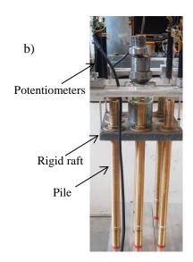
Figure 3. a) Raft model ; b) Piled raft model
