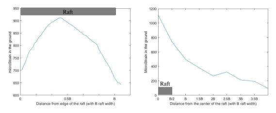
Figure 10. Deformation measured under the raft base
