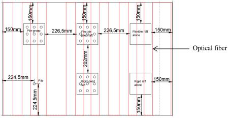
Figure 4. Optical fiber implementation plan
