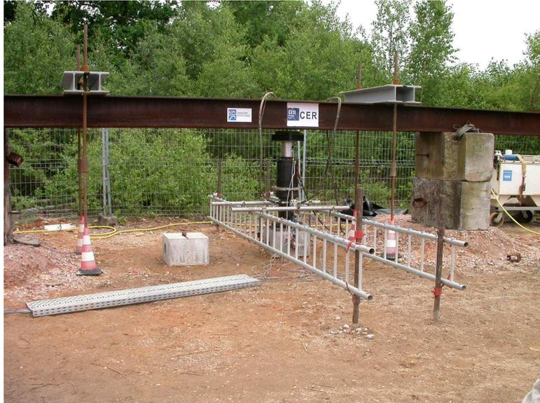
**Fig. 7 Photo of the pile load test system**
