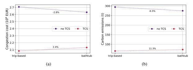
**FIGURE 10**: Variations of the objectives measures between bathtub and trip-based MFD: (a) congestion cost (total schedule cost) and (b) carbon emission.
