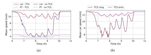
**FIGURE 7**: Effect of the different dynamic TCS of the mean traffic speed: (a) mean car and PT speeds with dynamic TCS ('mid') and without TCS and (b) mean car speed for the TCS 'cong' and 'emis'.
