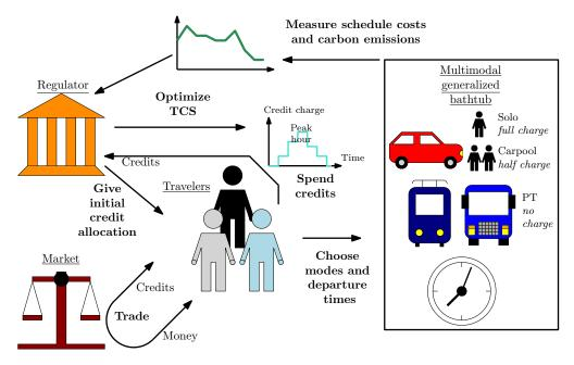
FIGURE 1: Framework of the multimodal bathtub under TCS.
