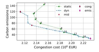
**FIGURE 5**: Congestion cost vs. carbon emissions for different static and dynamic TCS. The numbers are the ratios charge over allocation for the static cases. For comparison, the no TCS case leads to a congestion cost of  $2.63 \times 10^{6}$ EUR and a carbon emission of 275 t.
