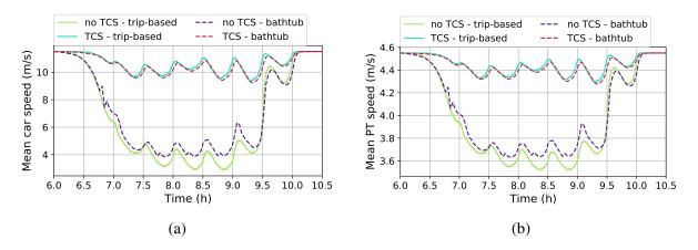
**FIGURE 9**: Comparison of the mean speeds with and without TCS for the bathtub and trip-based MFD resolutions: (a) car and (b) PT.
