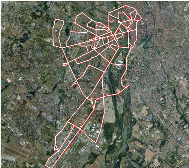
Figure 5 - Ultimate reference trajectory : almost full coverage, accuracy < 50cm, 100Hz
