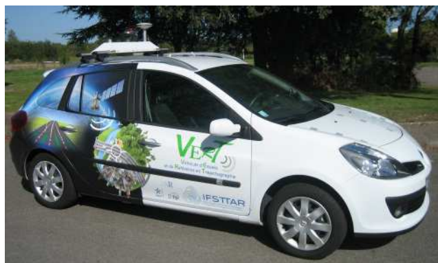
Figure 1: the Ifsttar Vehicle for Experimental Research on Trajectories and the iXSea IMU
