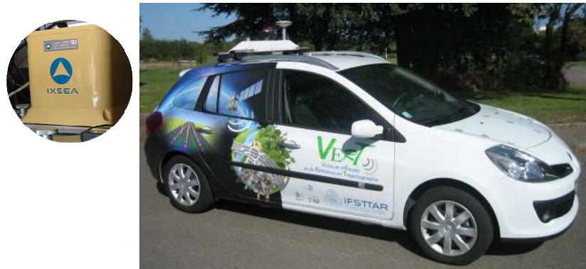
Figure 1: the Ifsttar Vehicle for Experimental Research on Trajectories and the iXSea IMU
