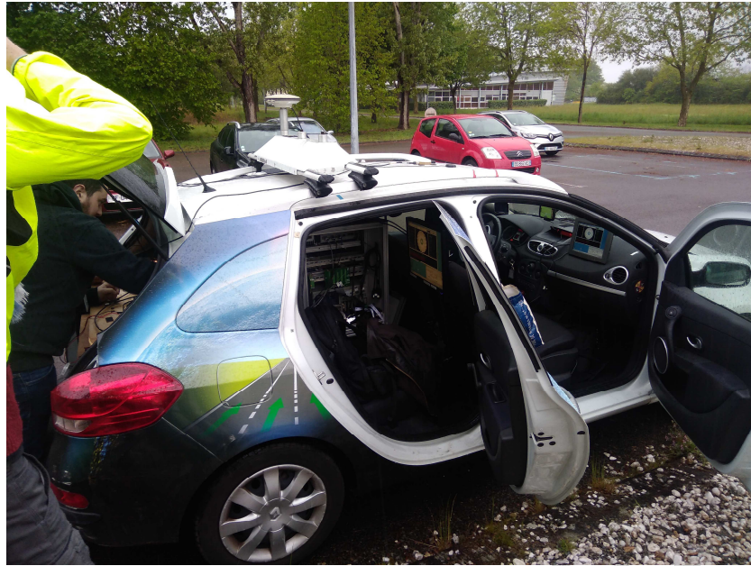
Figure 2 – Antennas on the roof top of the VERT
