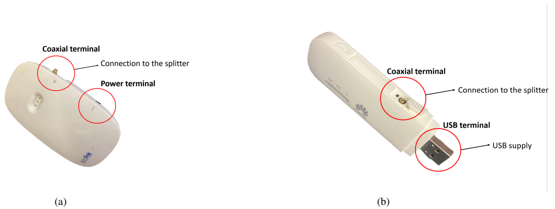
Fig. 6. Illustration of the power supply and coaxial connections. (a) Gateway. (b) LTE user device.
