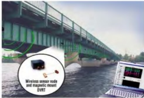
3. Wireless sensors are used to measure long-term stress and strain in civil engineering structures like buildings and bridges. (Courtesy: Microstrain Inc.)
