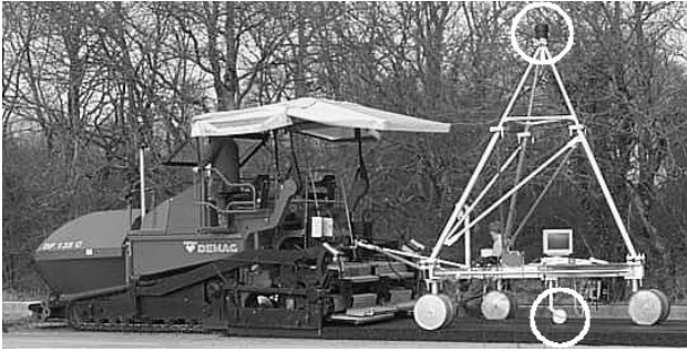
Figure 1: A CIRPAV demonstration: the LASERGUIDE is mounted on a trolley drawn by the asphalt paver and equipped with an encoder wheel
