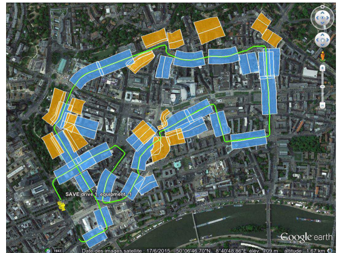
Figure 8: Virtual gantries designed in our experimental area in Frankfurt: the reference trajectory crosses through 20 virtual gantries
