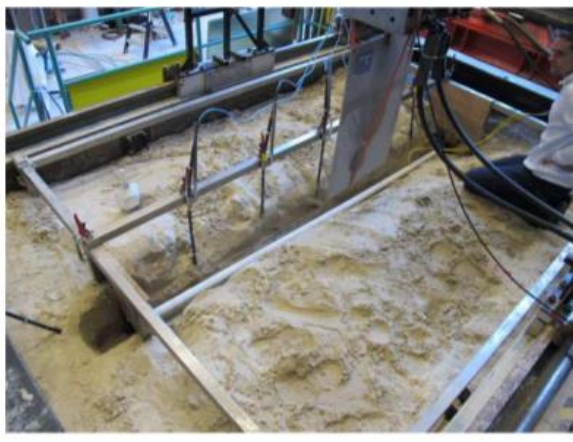
1. Placement of the pile in the model container. The diameter of the HDPE pipe was 50 mm with a wall thickness of 4.6 mm. The pipeline was laid 200 mm below ground level and at 150 mm from a sheet pile wall.
