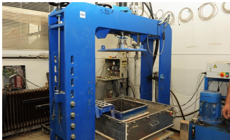
Figure 5 Set-up for friction test between two types of submerged geomaterials
