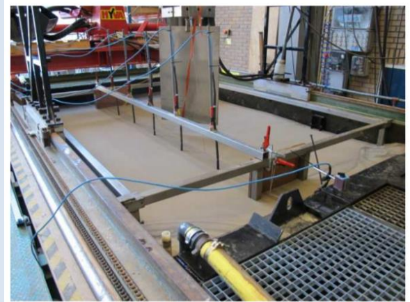
2. Sand has been carefully applied on top of the pipe. Before the start of the trial, a homogeneous loosely packed sand was prepared. This is done by fluidizing the sand (flowing upwards by means of water supplied from underneath over the entire bottom). In this way a sand package with a relative density of approximately 25% is obtained. The vertical and horizontal displacement of the ground was measured using Shape Accel Array Filed sensors.
