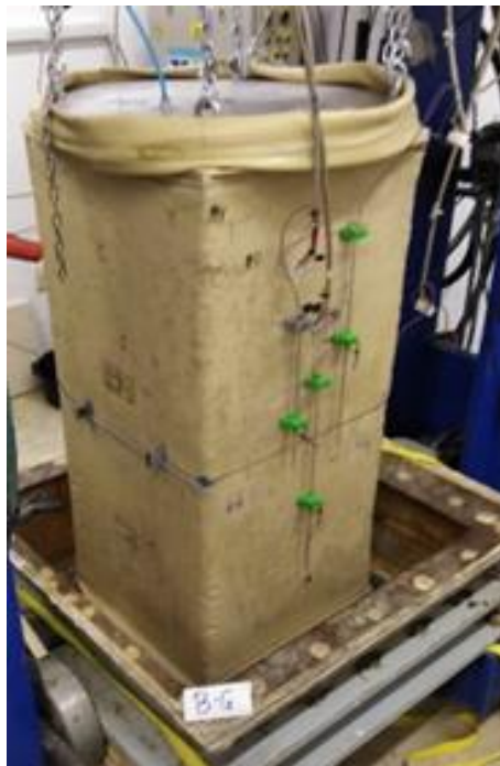
Figure 8 Prismatic specimen for triaxial test. Local LVDTs attached on side.
