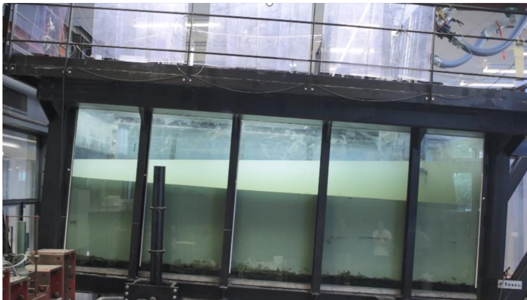
Figure 39. Liquefaction tank during tilting with a uniform seabed [Maghsoudloo et al. 2018, 2017, De Jager et al. 2017, De Jager 2018]
