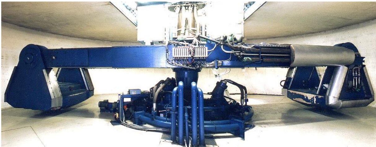
Figure 26 The 9 m diameter 500 gton capacity KRUPP geotechnical beam centrifuge (photo from Bochum).
