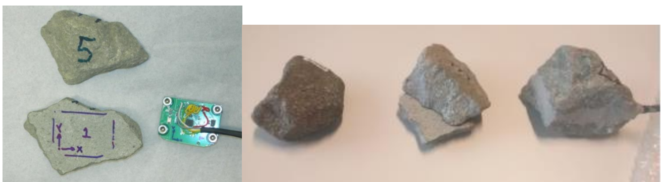
Figure 3-15 Ballast particles instrumented with accelerometers
