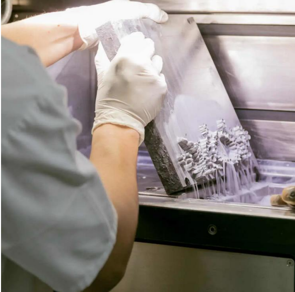
Figure 4-3 Removing a finished SLS 3D printed part (Ultimaker, 2022)
