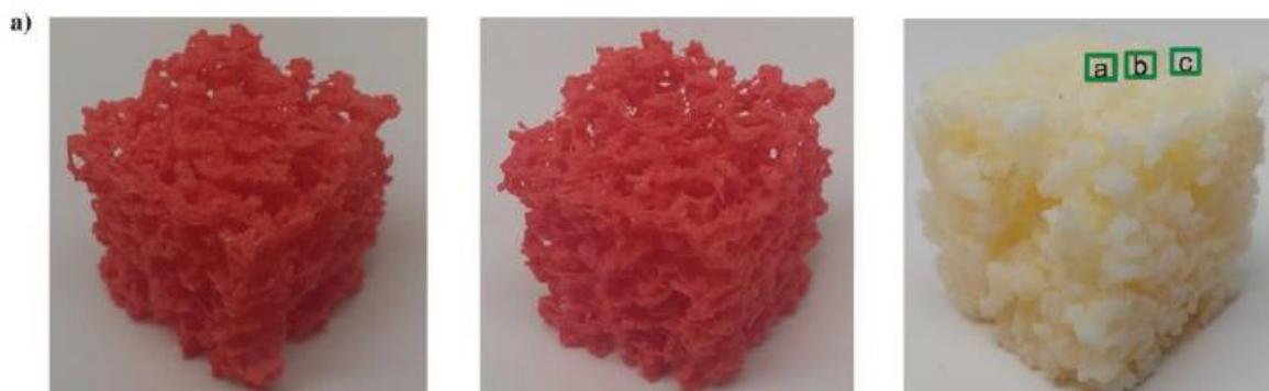
Figure 4-45 Networks of fractures obtained from 3D printing by the FDM technique (from Ishutov et al., 2014).
