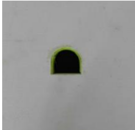
Figure 4-50 Scale model built by 3DP of a tunnel. The block is printed with a gypsum-based material, and the coating is PLA (from Song et al., 2018).
