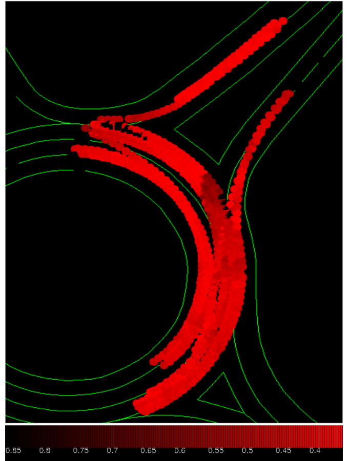
Fig. 7. Errors between the yaw angle estimated from RTK GPS positions and from the camera, in radian.
