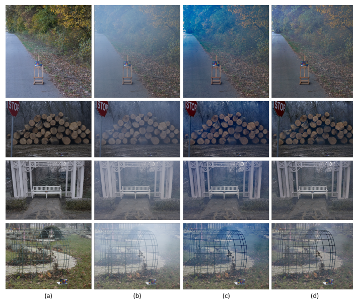
Figure 15. O-HAZE images [40]: (a) without fog, (b) with fog, (c) images restored with the White fog version of our algorithm (W), (d) images restored with the color version of our algorithm (C).
