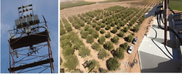
Fig. 2. Photographs of the experimental site and the antenna array at the top of the tower. The seven small antennas in the top frame are those operating in the C-band.
