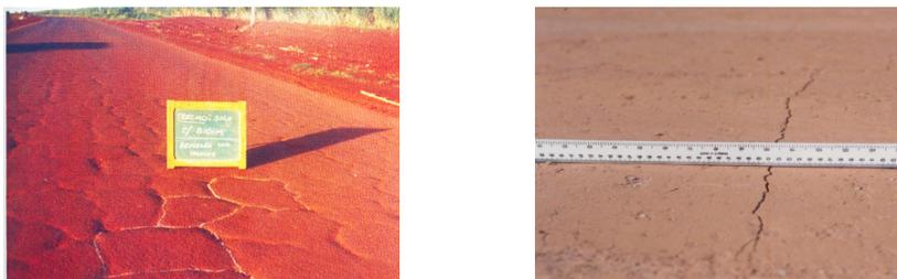
**Figure 3.** Cracking on pavement made of fine and coarse lateritic soils [VIL 09].
