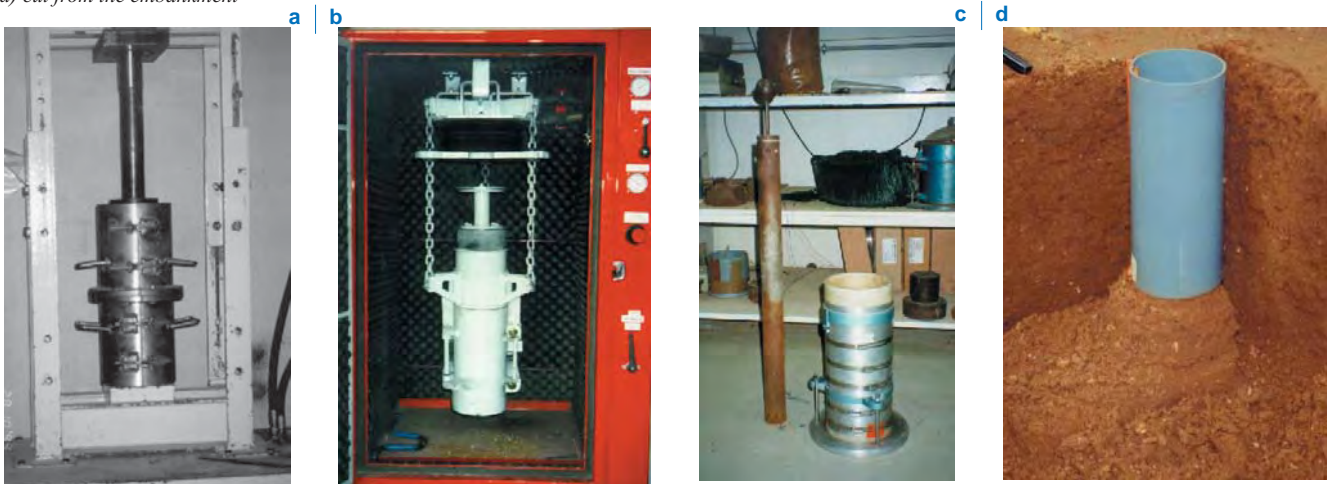
figure 10 Recomposed specimens by means of: a) static compaction; b) vibratory compression; c) the Proctor hammer; and d) cut from the embankment
