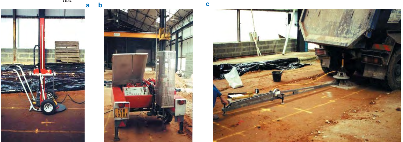
figure 11 Measurements performed on the embankment: - a: using the dual probe, - b: with the dynamic penetrometer, - c: by running the plate test
