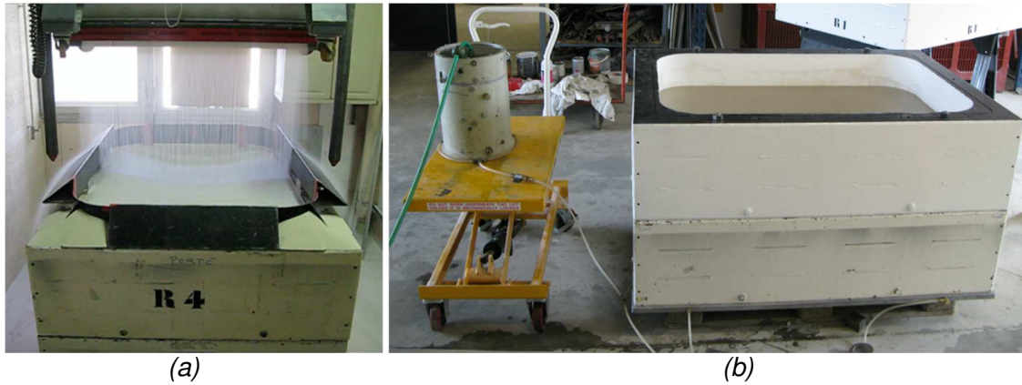
Figure 3 Preparation of the sand specimen: (a) pluviation; (b) saturation
