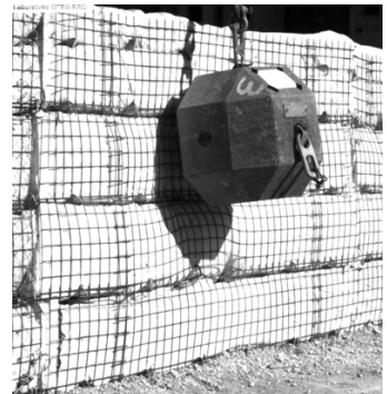
226 227 Figure 4. Embankment 1 deformation at the end of: a) the first phase; b) the second phase; c) the third phase. 228
