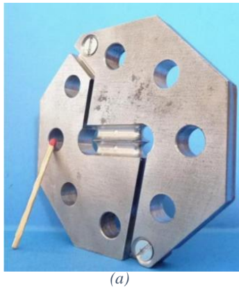
FIGURE 2 - (a) Arcan test TCS developed by Créac'hcadec et al. [6], (b) Zoom on the Arcan TCS beaks [6]
