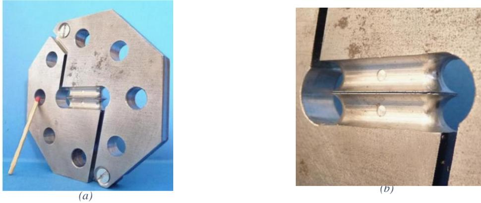
FIGURE 2 - (a) Arcan test TCS developed by Créac'hcadec et al. [6], (b) Zoom on the Arcan TCS beaks [6]
