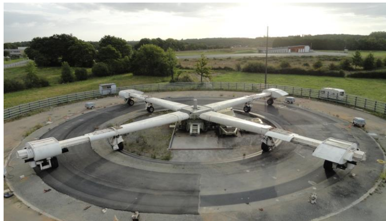
Figure 1. Full-scale accelerated fatigue experiment on asphalt pavements at Gustave Eiffel University in Nantes.
