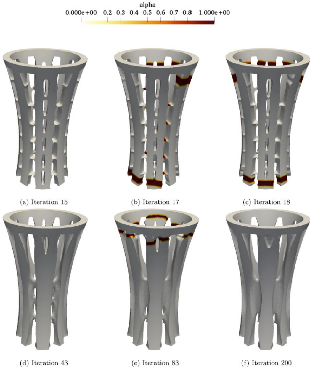
Fig. 13 Damage variable at the final time plotted for several optimization iterations (black regions indicate cracks). Reproduced from [163] with permission.
