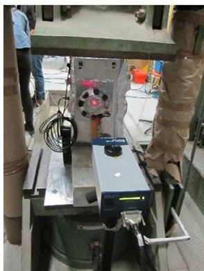
CWI and TREND methods on slab under compressive load
