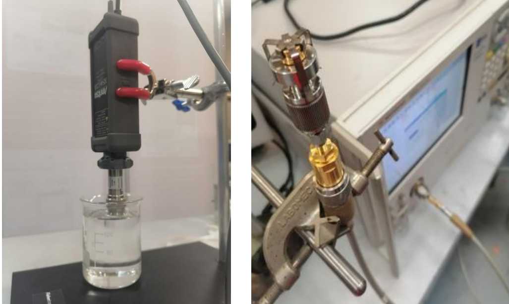
Figure 1: a. Measurement with Probe 1 b. Calibration with Probe 2
