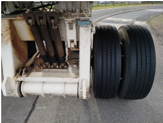
Fig. 2 a) Dual wheels of the carousel, b) Traffic density as a function of the lateral positions of the dual wheels axis per 100 000 loadings
