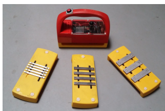
Figure 4: Capacitive measurements electrodes PE, ME and M3E as seen from left to right
