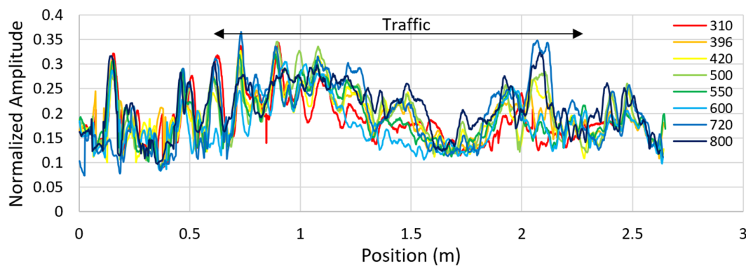
Figure 28. 2.6 GHz Normalized RW amplitudes on tack-coat free (I-3), in the transversal direction vs. K loadings.
