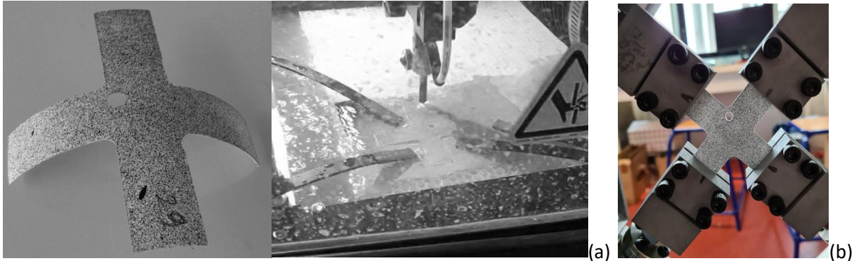
Figure 7: (a) Biaxial specimen with hole and speckle cut from bottle with water jet machine; (b) placed on biaxial machine with speckle.
