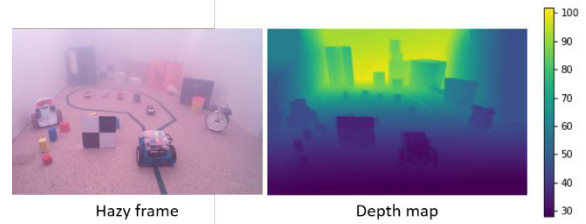
Fig. 2. Hazy frame and the associated false-colour depth map. Graduations are in centimeters.
