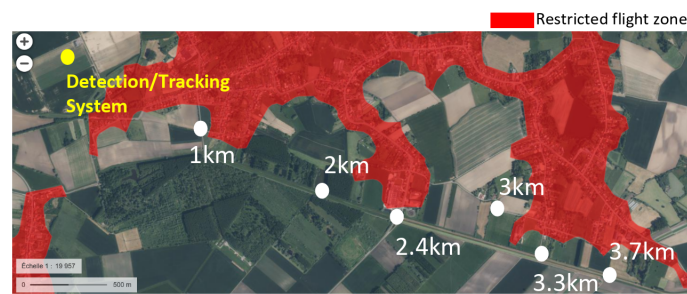
Figure 13. Outdoor mapping for long-distance drone experiments: system location (yellow spot) and pilot/drone positions (white spots).
