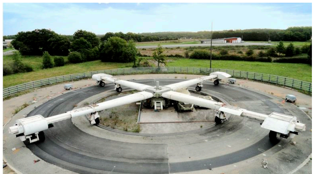
Figure 2. The pavement fatigue carousel at Univ. Eiffel Nantes [16].
