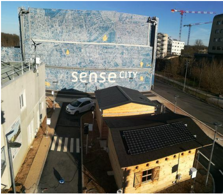
Fig. 3: The Sense-City facility. Foreground: urban scenario with 3 buildings and a drivable road. Background: mobile climate chamber.
