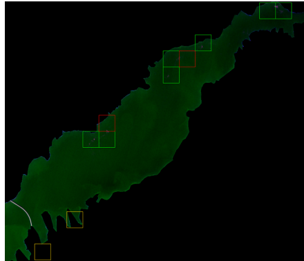
Fig. 9 Oil spill map of a Balkan lake. With green the successfully identified oil spills. In red the missed oil spills. With yellow the false positives.
