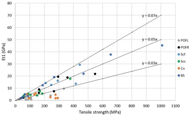
**Figure 8.** Modulus of elasticity vs tensile strength.
