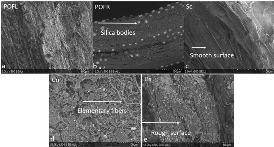
**Figure 3.** SEM images of external aspects of POFL (a), POFR (b), Sc (c), Cn (d), and Bs (e).
