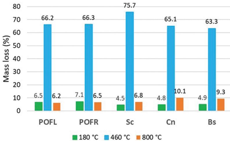
Figure 5. Mass loss of fibers with heat.
