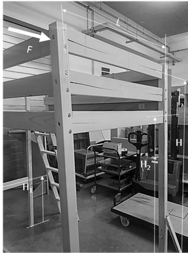
Fig. 10. High loft bed after testing at FCBA: the three upper bed rails show horizontal crack propagation, while the fourth lower rail is completely broken and is laying on the side of the right bed post. All the geometric dimensions in the vertical direction (namely the heights H , H_1 and H_2 ) are measured from the floor.
