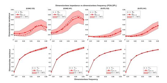
Figure 2: Dimensionless impedance vs dimensionless frequency (resistance top and reactance bottom). For  $\mathbf{W} = \mathbf{w}_{\mathrm{O}}$  with  $\mathbf{w}_{\mathrm{O}} = (\mathrm{POA}_{\mathrm{O}}, \mathrm{SPL}_{\mathrm{O}})$ , CAA ( $R_{\mathrm{O}}$  and  $V_{\mathrm{O}}$ ) (black broken lines), conditional expectation ( $\underline{R}_{\mathrm{PLoM}}, \underline{V}_{\mathrm{PLoM}}$ ) from PLoM (red line), and 98% CI from PLoM (red zone).
